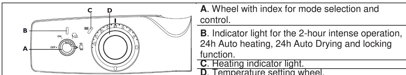
Switching on and setting the correct heating temperature. The device is designed for heating the room and establishing a comfortable temperature.
