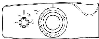
In the example given above, in which the calibration value was  $-1^{\circ}\text{C}$ , it just so happened that the end position of the wheel was beyond the symbol. The device will maintain a temperature of  $7^{\circ}\text{C}$ .
